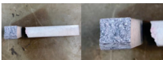
Fig. 9. Crack propagation in Izod V-notch specimens
