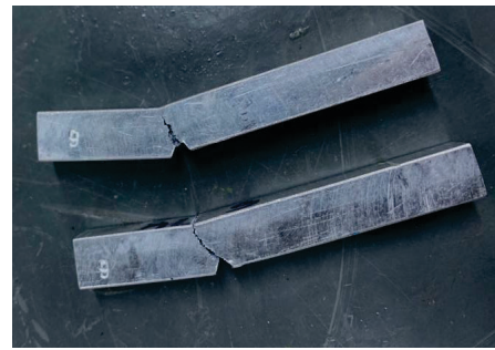
Fig. 10. Crack propagation in Izod V-notch specimens of ETIAL 195
