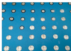
Fig.5. Compression EH mounted on a pedestrian power generator walkway.
