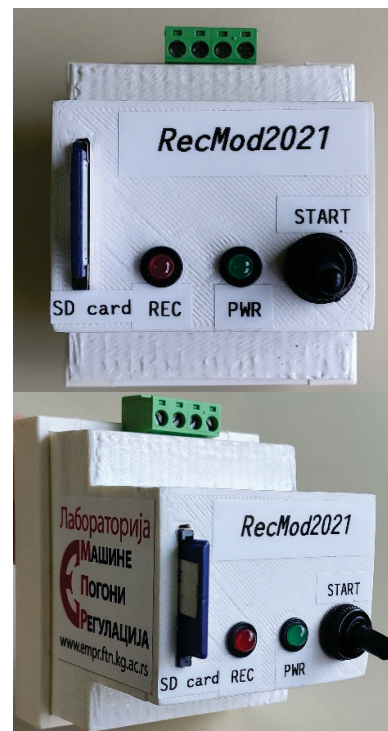
Fig. 4. Final look of the developed RecMod2021 device - ver. 1
